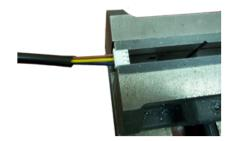
3. GRASP THE BROWN WIRE GENTLY, AND WHILE PUSHING IN, DEPRESS THE METAL TAB WITH A FINE POINTED TOOL.
