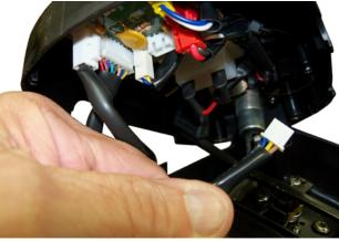
5. Remove the two Phillip screws holding the throttle on the tiller
