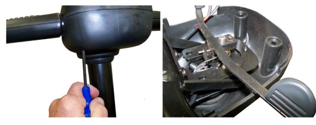
4. Locate the wires from the throttle and disconnect.
