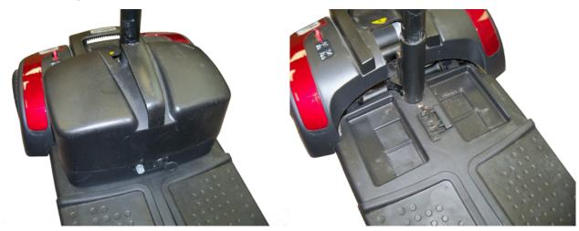
2. Locate the four Allen head screws holding the top and bottom of the tiller cover together.
