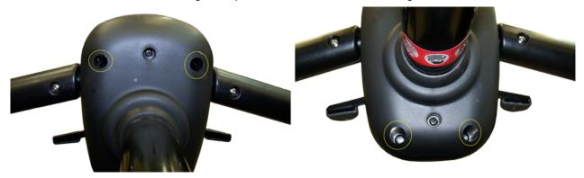
3. Remove with a 4 mm Allen wrench and separate the two halve of the tiller cover. They will not come completely apart because of the wiring inside of the tiller cover.
