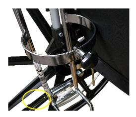
9. When an O2 cylinder is placed in the O2 holder it must be locked in place by turning the cylinder locking knob clockwise.
