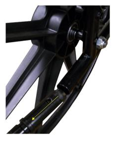
3. Remove the cap screw from the U bracket and slide the unit onto the left side frame. If the unit will not slide unto the left side frame remove the spacing sleeve. Continue sliding the unit onto the left side frame until the U bracket wraps around the rear upright of the left side frame.
