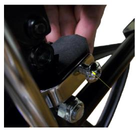
5. Tighten with a metric Allen wrench.
