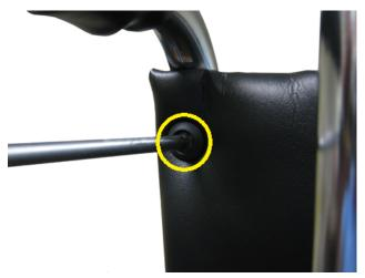
8. Insert the backrest screw through the offset bracket and reinstall the screw in the chair.
