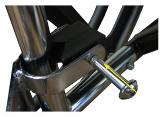
6. Tighten with a metric Allen wrench.
