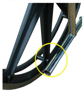
3. Remove the cap screw from the U bracket and slide the unit onto the left side frame. If the unit will not slide unto the left side frame remove the spacing sleeve.
