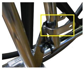
5. Slide the cap screw thought the non-threaded side of the U bracket and the spacer bracket.
