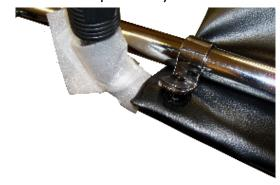
6. Tight the screw. The IV pole is now installed.
