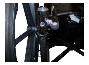
3. Install the tipping sleeve or anti-tipper.
