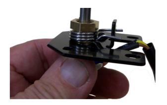
9. Tighten the throttle spring retaining nut with a wrench.
