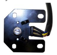
4. Slide the new throttle spring down over the throttle pot with the bent end as shown.
