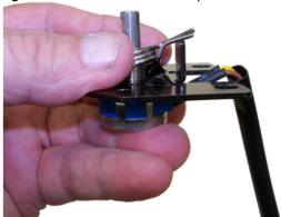
5. Place the bent end on the side of the throttle spring stop. Push the other side of the throttle
