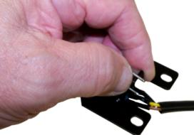
6. Push the throttle spring down flush with the throttle mounting bracket.
