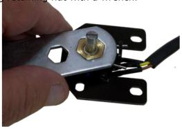
10. Install the throttle lever Allen set screw.
