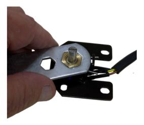
3. Remove the defective throttle spring.
