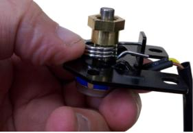
8. Hand tighten the throttle spring retaining nut down to the throttle mounting plate.
