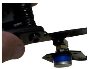
2. Remove the throttle spring retaining nut.
