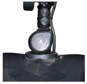
2. Pull out the tiller locking knob and turn to the upright position. If there is any difficulty in pulling out the tiller locking knob turn the tiller slightly either left or right untill the tiller locking knob can be pulled out.
