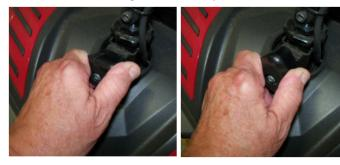
3. The tiller is unlocked when the tiller release knob is in the upright position. To lock the tiller reverse this proceedure.
