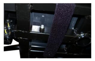
4. While holding the head of the bolt against the frame, use a 13mm wrench or socket to remove the nut.
