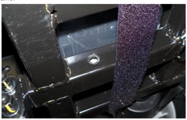
6. Slide the footplate mounting plate forward and align the rear mounting hole with hole in the frame.
