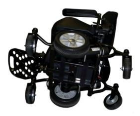
2. Using a #3 Phillips screw driver to remove the lower front shroud.
