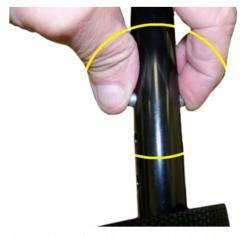
4. Turn the footplate slightly, slide to desired length and engage the double push button.
