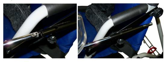
12. Making sure that both sides of the tray are equal distance from the arm frame, tighten the set screw in the tray bracket.
