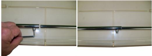
4. Remove nut from upper armrest attachment point. Leave the washer in place on the threaded rod.
