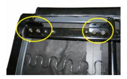
3. Position the TRID-2A40 ELR adapter on seat frame of the chair. Using four screws from the seat brackets previously removed; loosely thread them through the adapter plate to the seat frame.
