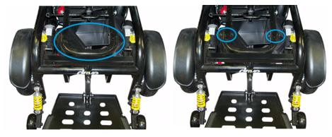
4. Slide one of the "T" brackets from the SFELR kit into the TRID-2A47 bracket with the welded nut facing up. Lock the "T" bracket in the TRID-2A47 with either the provided cap screw and nut or a grenade pin. The use of the grenade pin facilitates easy adjustments.
