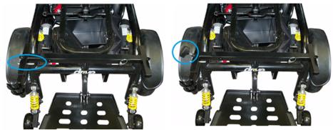
8. Repeat for the left side. Now the Trident is able to use a set of footrests or ELRs. Adjust the brackets as needed. Install the seat back onto the Trident.
