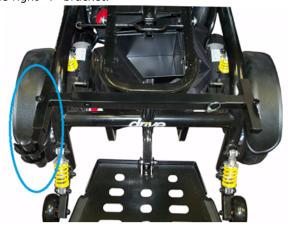
7. Slide one of the grenade pins through the "T" bracket and the ELR bracket. Install one of either the Allen head set screw or a locking knob to lock the ELR bracket in place. The use of the locking knob facilitates easy adjustments.
