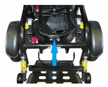
3. Install the two button head screws through the TRID-2A47 bracket and the upper frame. Thread the nut onto the button head screw and tighten.
