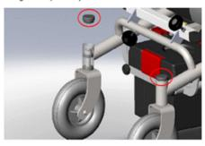
2. Remove the two M12 nuts securing the caster forks to the frame with a 19mm socket wrench
