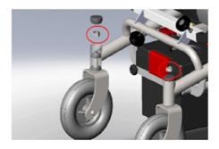
Using the washers supplied, install one washer per caster fork as pictured below (washer is highlighted in yellow)
