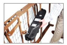
Align the opening on the foot end of the motor with the flange on the foot section of the bed and insert the flange into the motor compartment.
