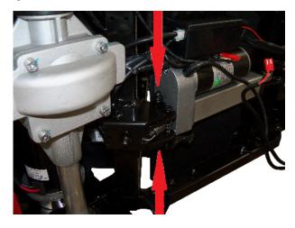
5. Grasp the yellow folding release rod and fold the unit about half way. This will disengage the actuator from the rear of the unit.
