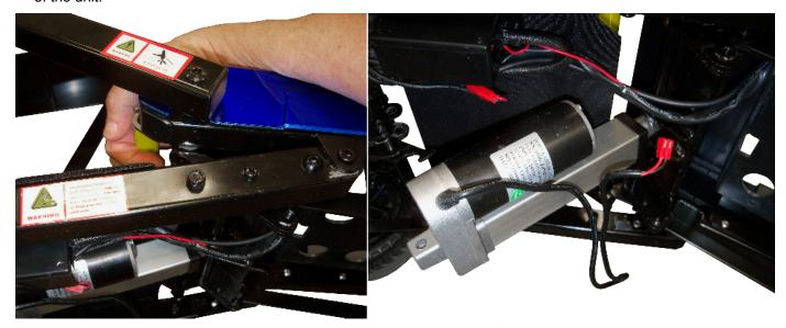
6. Remove the 2 "E" clips on the rod holding the rod that is inserted into the front of the actuator motor.
