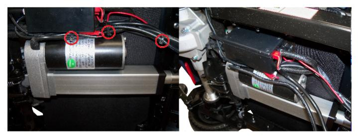
3. Unplug the actuator wire from the control box.
