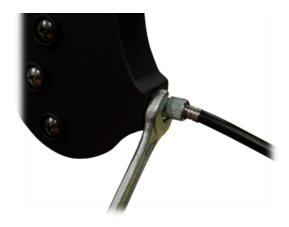
5. If further adjustments are need the same procedure can be made at the lower cable adjuster. Loosen the brake cable adjustment nut away from the frame.
