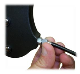
4. Tighten the brake cable adjustment locking nut against the brake handle housing.
