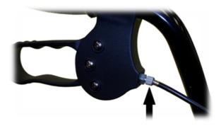
2. Loosen the brake cable adjustment lock nut away from the brake handle housing.
