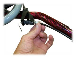
7. Tighten the brake cable adjustment nut against the frame.
