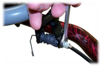
6. Turn the hand brake adjuster counterclockwise to tighten the brake or clockwise to loosen the brake.
