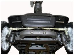
2. Locate the tie rod for the wheel that is toed in or out.
