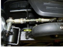
3. Place a wrench on one of the nuts and one on the tie rod. Loosen the nut. One of the nuts will be reverse threaded.
