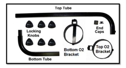
2. Slide the bottom tube into the top tube. Install one of the locking knobs into the top tube and tighten. Installing the bottom tube as shown will have the O2 tank on the right side of the seat. To have the O2 tank on the left side of the seat, flip the bottom tube 180 degrees and install into the top tube.
